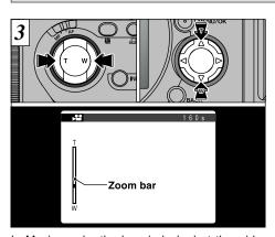
In Movie mode, the lens is locked at the wideangle setting and only the digital zoom can be used. You can use the Zoom button or the 4direction button "▲" and "▼" to zoom in and out. When you use the zoom, a "Zoom bar" appears on the screen.
